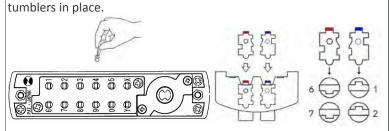
6. Replace the cover plate and secure with two (2) Red Screws, using a #2 screwdriver.
