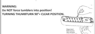
4. With the thumb-turn held 90° to right or left, remove/add CODE (Red) and NONCODE (Blue) tumblers to create the desired code.
