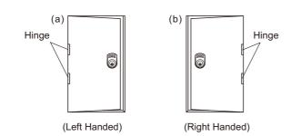
Note : When installing make sure the door opening side.
