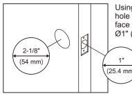
Using the marks as a guide to drill a hole Ø2-1/8" (54mm) through the door face for the lockset, then a hole of Ø1" (25.4mm) for latch.
