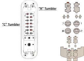
4. When completed changing your code, release the "C" button and replace the plate carefully.
