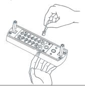
3. Code is made up of RED tumblers. Make sure the colored end is facing upwards. Example: If your desired code is 13569, red tumblers will be placed in numbers 13569 (shown below).
