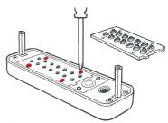
2. Hold the "C" button from underneath from now until you have completed the code change.
